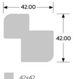
One universal profile for indoor and outdoor usage. Boards with straight-cut ends can be installed without exposing the endgrain.
