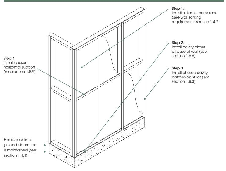
Once the wall has been battened out as per cavity construction details, Weathertex's product specific standard fixing instructions shall be followed to install the cladding on to the frame.
