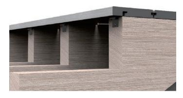
5. Install the starting clips at the top of the vertical face of the joist.
