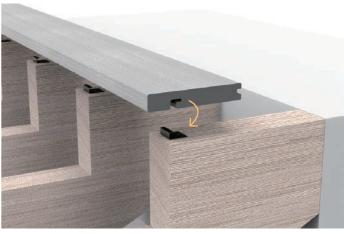
2. Install the edge board onto the starting clip.
