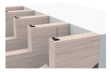
1. As shown in the diagram above, determine the position and install the starting clip.
