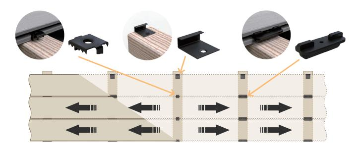
STARTING CLIPS LOCKING CLIP SPACING CLIPS 13 per board (1 on every joist) on the first run of decking only
