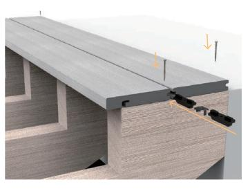
4. Insert the clips along the groove between the two boards, sliding into the correct position above the joist, before fixing. Rip the back edge of the secondary board to suit the depth of your tread. Fix the back edge with a face screw.
