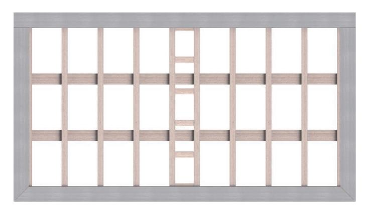
PICTURE FRAMING METHOD OF DECKING INSTALLATION - INSTALLING THE CLIPS
