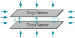
Structural "A" bonds require rigorous testing after submersion in boiling water for 72 hours or 6 hours under high pressure steam to ensure a high quality bond.
