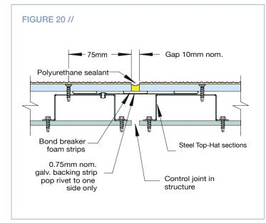
Module slip/control joints over CFS Top-Hat framing must have a 10mm gap between each adjacent module of Duratex<sup>™</sup> panels, as shown in the diagram below.
