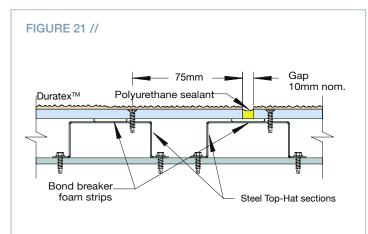
Horizontal joints are similar to the vertical jointing systems and may be expressed or have architectural details applied.
