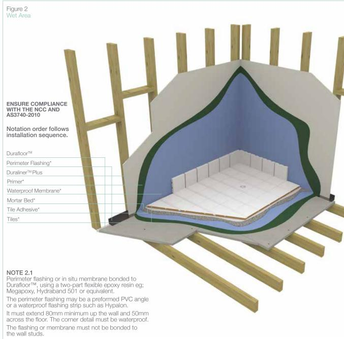
An additional wall nogging must be installed so that the bottom of the Duraliner™ Plus is fastened above the perimeter flashing.
